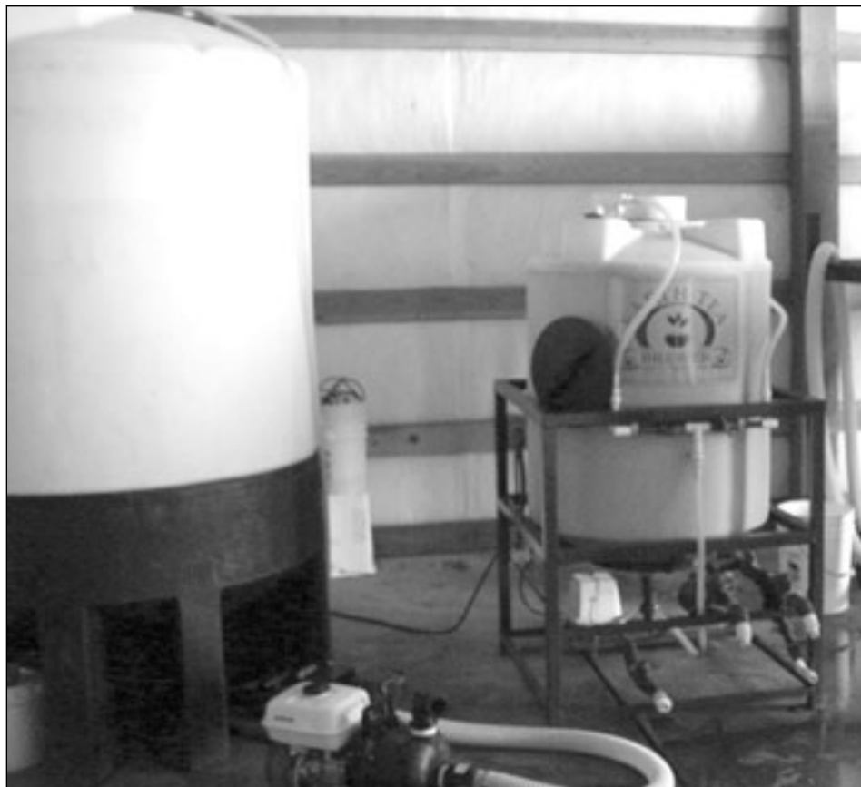
A 100-gallon EPM tea brewer in action at Soil Smith Services in Philomath, Oregon. Excellent fungal, bacteria and protozoan numbers can be achieved with this machine.
