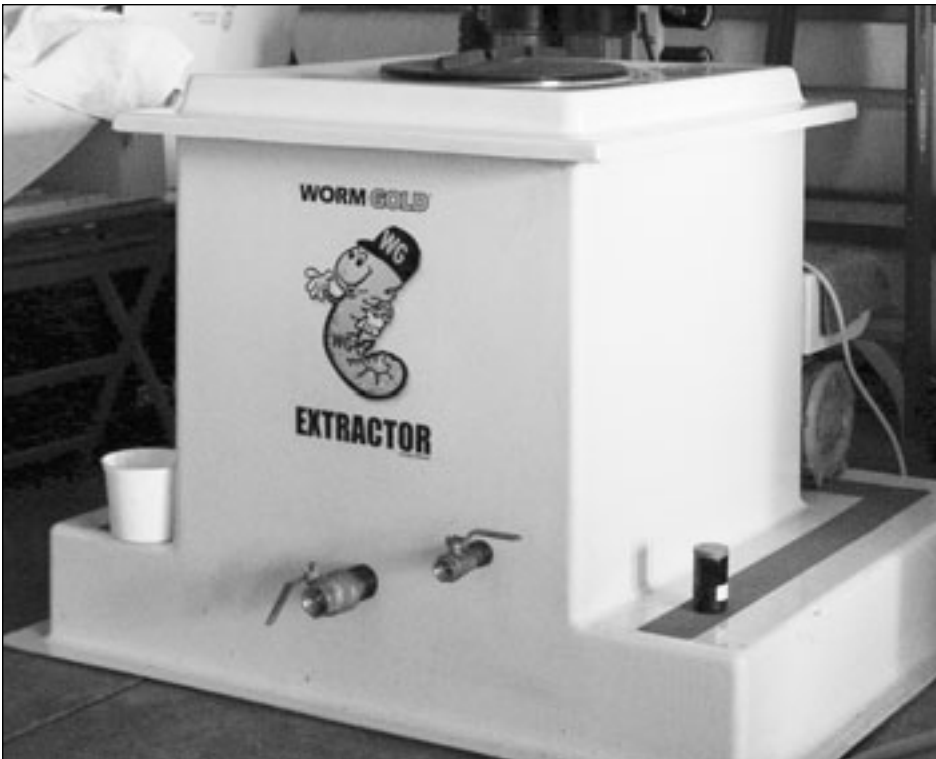
A 50-gallon WormGold machine at Soil Smith Services in Philomath, Oregon. Very consistent, high fungal, bacterial and protozoa tea can be produced with this machine. Data for this machine is available on the WormGold website < www.wormgold.com > showing the consistent quality of their tea.
