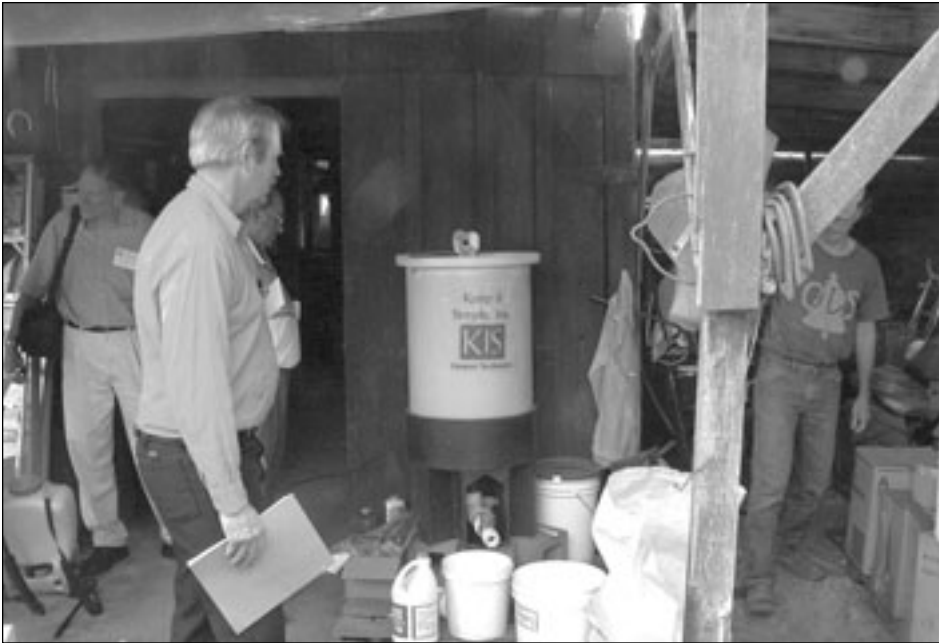
A 28-gallon KIS brewer in action at a local farm near Corvallis, Oregon. Excellent tea with high biomass of bacteria, fungi and protozoa is consistently produced with this machine. Data for this machine can be found at < www.simplici-tea.com >.
